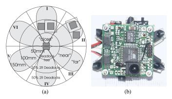
Figure 2: (a) Problem of IR-interferences in the "close", "near" and "far" communication zones; (b) The sensors board with Megabitty board that supports 6-x directional robot-robot and host-robot communication, proximity sensing and perception of surfaces geometry.
