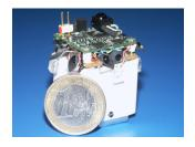
Figure 3: The prototype of the "Jasmine" microrobot.
