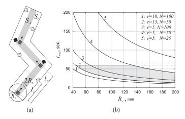
Figure 1: (a) Motion path of a robot with communication and collision-avoiding contacts; (b) Total propagation time  $t_{total}$  as a function of communication distance  $R_c$  with different values of velocity v and the number of robots N.
