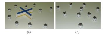
Figure 6: Preliminary experiments with 10 microrobots; (a) Collective perception; (b) Building a "communication street".
