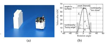
Figure 7: (a) Scanning of the finite-size surface; (b) The IR-diagram for finite-size surface and the used features of IR-diagrams relevant for identifying the surfaces.
