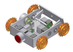
Fig. 1. CAD design of a wheeled module with bending capability and rotational degree of freedom; docking mechanisms (not shown in the picture) are placed on each sides.
