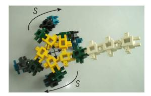
Fig. 11. Top-down view on the unsymmetrical scorpion, central modules (yellow) built a ring. Deforming this ring, different movement of legs can be created.
