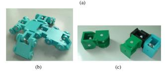
Fig. 6. Topological models of different modules. (a) (left) First rapid-prototyping model with docking elements and individual locomotion, (right) topological model of the PUZZBOT; (b) Topological models of wheeled modules; (c) Topological models of different crawling modules with 1.5 DOF and 3 DOF.
