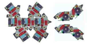
Fig. 3. Deflection of side docking connectors( $\pm 35^\circ)$  and back docking connectors( $\pm 45^\circ).$
