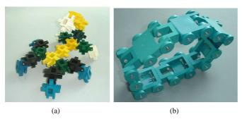
Fig. 7. Examples of "typical" macroscopic locomotion. (a) Legged scorpion-like organism; (b) Macro-wheeled locomotion of the organism.
