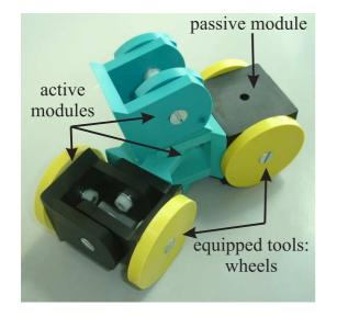
Fig. 9. "Car"-like organism, consisting of heterogeneous modules.
