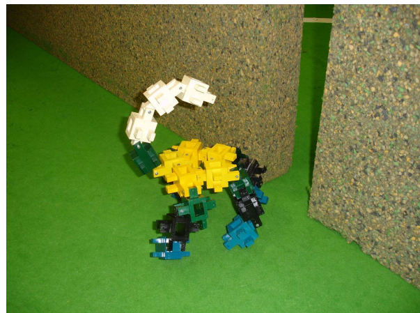
Fig. 6. The gap in a wall can be detected by local sensors (a topological model is shown). However, no information is available regarding the situation behind the wall. It means that the local fitness of some structural configuration may be very high before the wall, but it can get very low after passing the gap.
