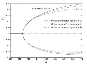
Fig. 3. Bifurcation diagram of the unstable mode of the mode equations (23) and the order parameter equation (40) with a quadratic and cubic center manifold. The order parameter 1 is obtained with the cubic center manifold, the order parameter 2 — with the quadratic center manifold and the order parameter 3 is based on the adiabatic elimination procedure.
